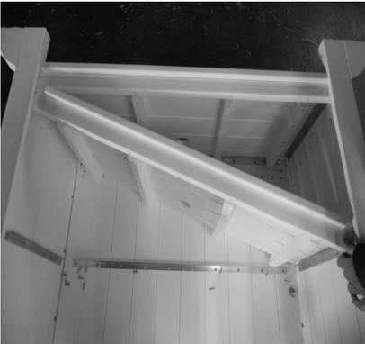
Insert middle shelf into bar at an angle as shown (Left Picture). Then place onto aluminum supports. Secure using (15) 3/4" Pan Head Screws through aluminum into shelf slats while holding legs tightly to the shelf. (Right Picture). Repeat process for bottom shelf.
