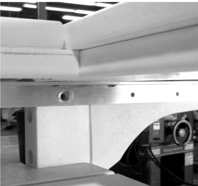
Stand up base assembly. Align long aluminum support on bar top with insert nuts on front legs of base assembly (Left Picture). Secure long aluminum with (2) 1" Phillip Pan Head Bolts (Right Picture). Then secure long and short aluminum supports using (12) 3/4" Pan Head Screws.
