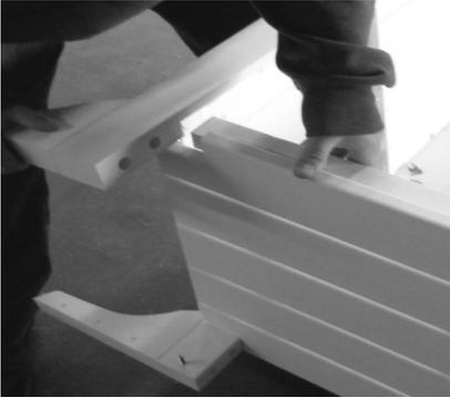
Place top shelf onto top aluminum shelf supports on front and side panels while lightly separating back legs just enough to fit shelf into pocket in legs (Left Picture). Secure using (15) 3/4" Pan Head Screws through aluminum into shelf slats while holding legs tightly to the shelf. (Right Picture)
