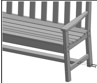
Align counter-bored holes in lower side stretcher with Pilot holes in long stretcher, making sure that the aluminum in the long stretcher is facing down. Attach using (2) 80mm Hex Lags. Plug holes with (2) 5/8" Bungs using rubber mallet.
