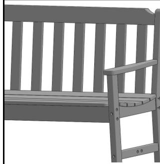
Align counter-bored holes in Rear Left Leg with Pilot holes in Back Assembly, ensuring that the
