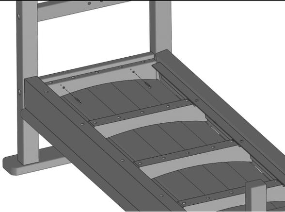
Secure outer seat cleat to side assembly using (2) 1-1/4" Phillips Head Screws.
