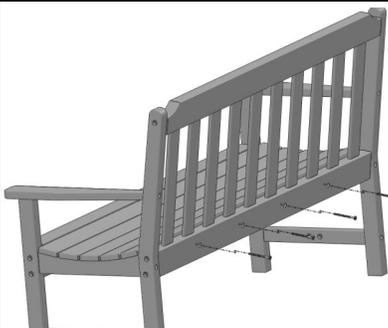
Secure Lower Back Assembly to Seat Assembly using (4) 80MM Hex Lags (3 for 037) thru counter-bored holes in lower back into pilot holes in seat supports. Plug holes with (4)
