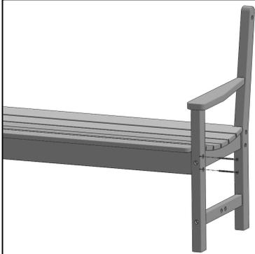
Align Left Side Assembly with seat assembly. Secure using (2) 80MM Hex Lags through the counter-bored
