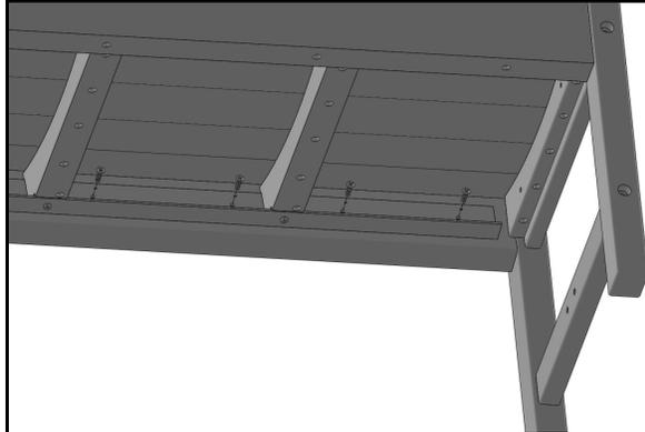
Turn Assembly upside down. Secure aluminum seat cleat to lower back using (9) 3/4" Phillips Pan Head Screws.
