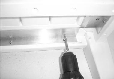
Attach Lower Shelf Apron Aluminum, which is pre-assembled on Leg Assembly to Shelf using (3) 3/4" Pan Head Screws. (Left Picture) Repeat process on other side.
